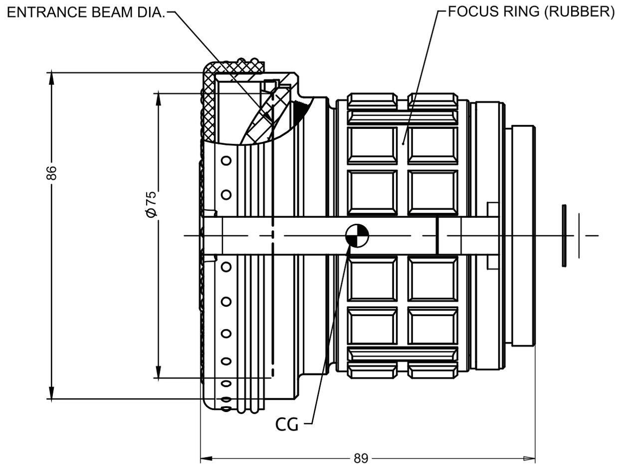
**PLEASE NOTE:** The drawing provided here is primarily a representation and may not accurately reflect the product's actual dimensions and specifications. For precise integration specifications, we recommend contacting your local sales representative.
