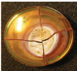
Fig. 4. Massive lens cracks, burn marks due to Beam Mode failure
