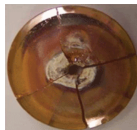
Fig. 6. Lens hole and coloration caused by oil contamination
