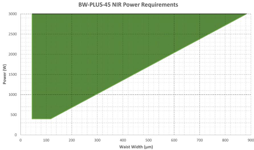
Figure 3: Minimum Linear Power Density in the NIR Range
