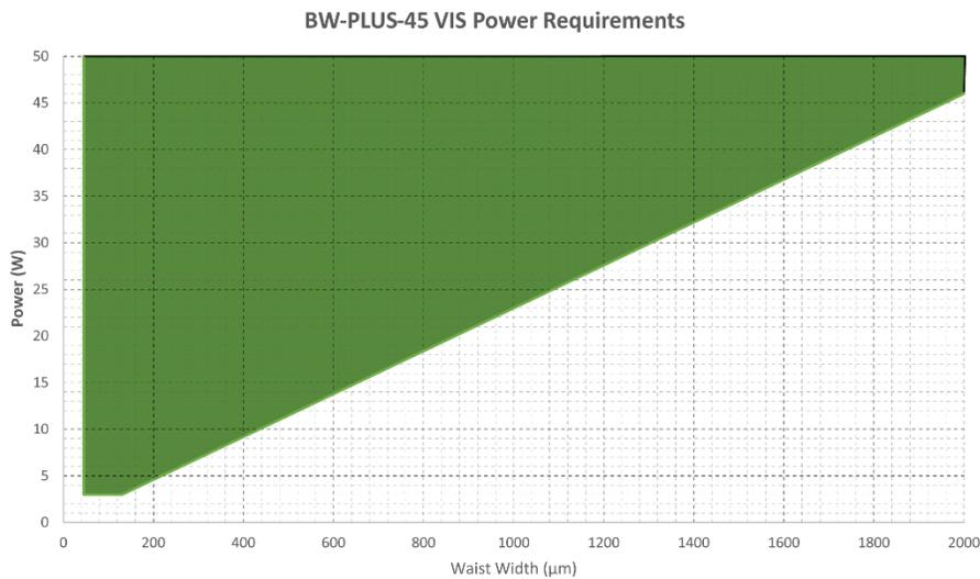
Figure 4: Minimum Linear Power Density in the VIS Range
