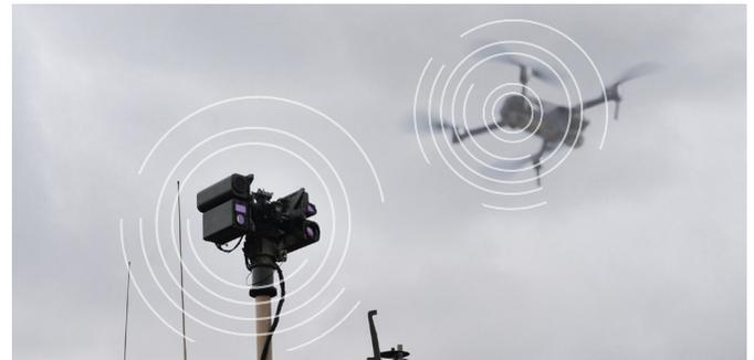
Fig. 1. C-UAS system using a combination of electro-optical and infrared sensors.
