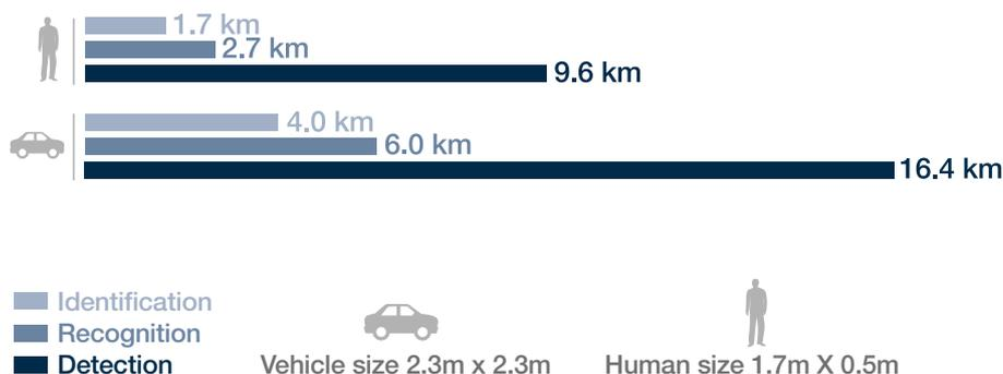
Assumptions: 10 $\mu$  pixel pitch | 3.6 $\mu$ -4.9 $\mu$  spectral band | 23mK NETD | 30Hz frame rate | 0.2km<sup>-1</sup> atmospheric attenuation coefficient | 50% detection probability | Human target – 1.7x0.5m size, 5°C  $\Delta$ T | Vehicle target – 2.3x2.3m size, 2°C  $\Delta$ T.
